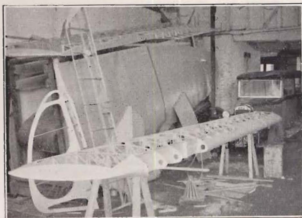
A new pair of wings under construction for the Kent Gliding Club's nacelled "B.A.C. I." In the trailer is the "B.A.C. VI."
