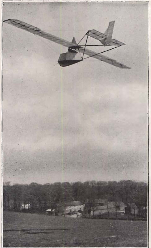
A scene at the Derbyshire and Lancashire Gliding Club: a nacelled "Dagling" is climbing on the winch cable, while in the background is Camphill Farm with the clubhouse.
