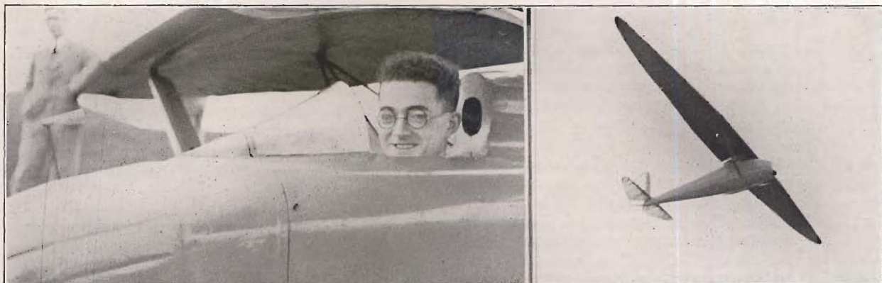
We do not know whether the low weight claimed for the "Merlin," illustrated above, is obtained by spring balance or by "guesstimation." But it can fly. Mr. W. E. Hick, of the Newcastle Gliding Club, its principal builder and designer, is seen in the cockpit. The span is 34 ft. 4 in., area 80 square feet, and wing section Göttingen 652.
